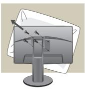
**2.** Separate the head and the stand with the use of a screwdriver.
